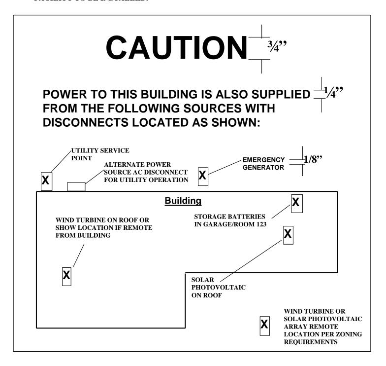
THE PLAQUE OR DIRECTORY SHALL BE METAL OR PLASTIC, WITH ENGRAVED OR MACHINE PRINTED LETTERS, OR ELECTRO-PHOTO PLATING, IN A CONTRASTING COLOR TO THE PLAQUE, AND SHALL BE ATTACHED TO THE SERVICE EQUIPMENT WITH POP-RIVOTS, SCREWS, OR EPOXY.
