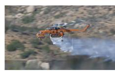
During fire season, our helitanker is available on short notice to help put out fires. It can carry and drop up to 2,650 gallons of water – more than seven times the 360-gallon capacity of a typical firefighting helicopter.
