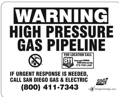
Pipeline markers indicate only the approximate, not exact, location of buried pipelines. Markers also do not indicate the depth or number of pipelines in the area. These yellow markers display the pipeline operator's name and a phone number to call in case of emergency.
