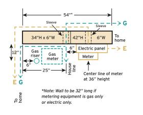
Note: Block wall specifications must meet all municipal codes. All voids in the blocks to be filled solid with concrete and contain minimum #3 rebar. Service sleeves for gas and electric house lines to be at 18 inches height.
