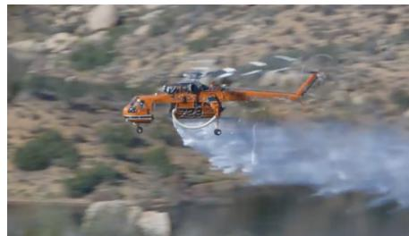
*During fire season, our helitanker is available on short notice to help put out fires. It can carry and drop up to 2,650 gallons of water - more than seven times the 360-gallon capacity of a typical firefighting helicopter.*
